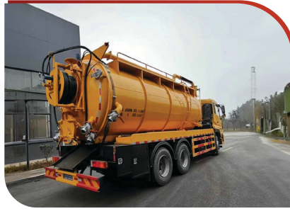
HIGH PRESSURE JETTING TRUCK
